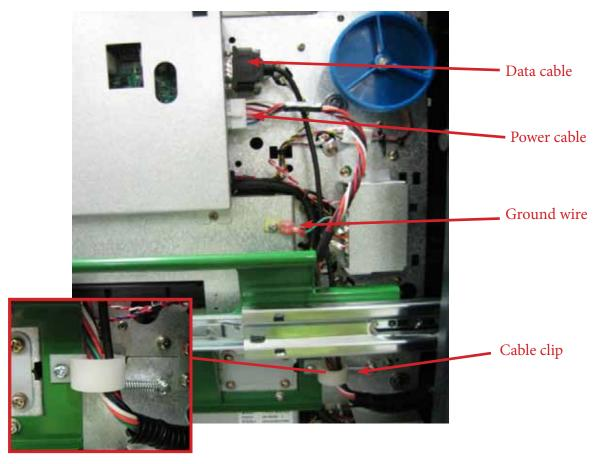
3. Grab the HCDU by the handles and lift it off the rails. Set the HCDU on the floor.
