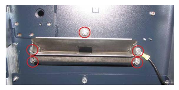
2. Disconnect the power cable, data cable, and ground wire from the HCDU. Remove the wires from the cable
