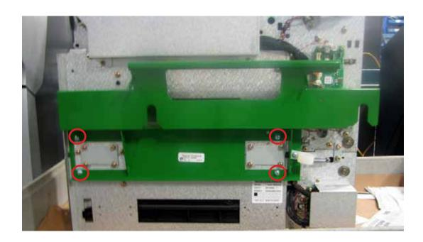
11. Gripping the HCDU by the handles, lift the HCDU. Set the HCDU on the rails with the standouts on the rails fitting into the notches on the handles.
