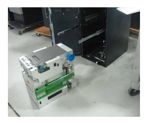
4. Remove the 8 screws (4 on each side) holding the handles in place.
