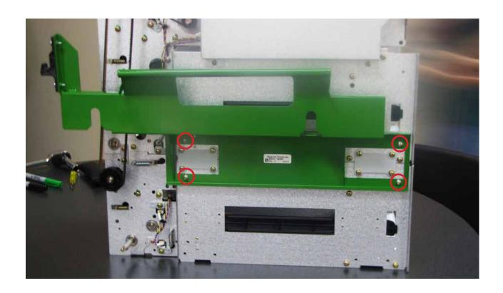
9. Obtain the new latch side handle and the cable clip. Install the cable clip on the latch side handle with the remaining #6-32/1/2" screw provided in the kit as shown.
