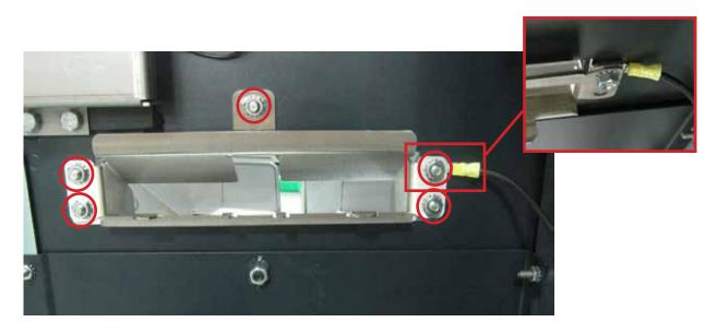
7. Obtain the new hinge side handle and part B of the bin latch. Install part B of the bin latch to the hinge side handle with 2 of the #6-32/1/2" screws provided in the kit. Make sure the hook is facing up exactly as shown.
