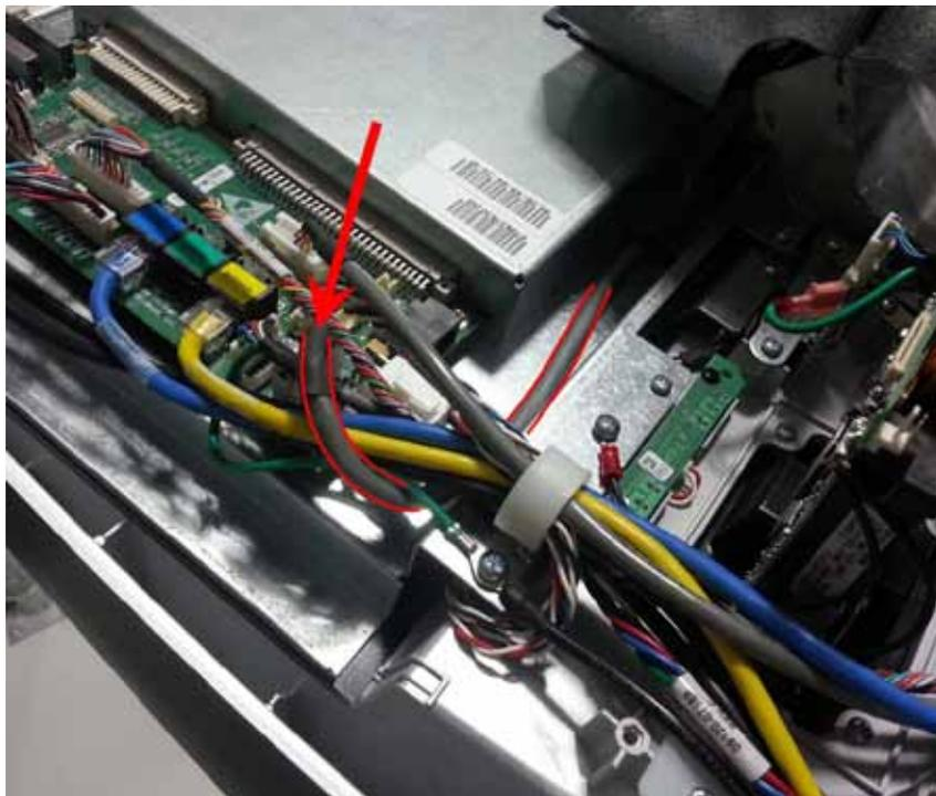
7. Reroute the printer power cable under the other wires and plug back into the docking board.
