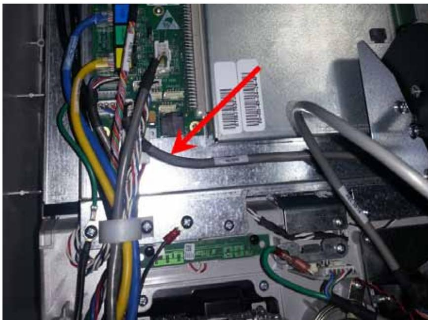
8. The slack will need to be taken out of the printer USB cable to allow room to install it on the new printer assembly. Take the slack out of the printer USB cable as shown.
