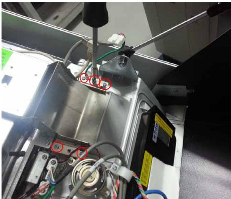
6. Unplug the printer power cable from the docking board.
