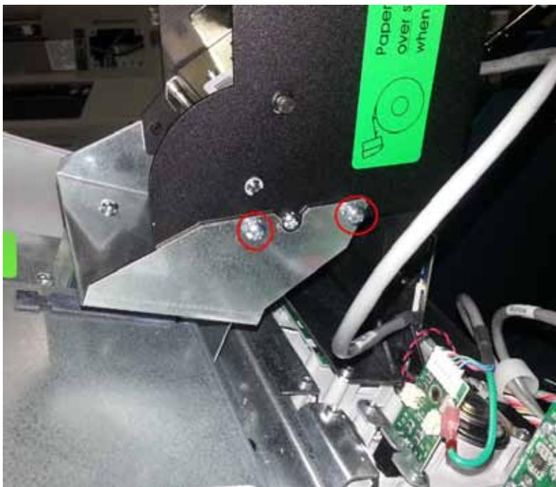
13. Install 2 nuts on the printer presenter, 1 on each side.
