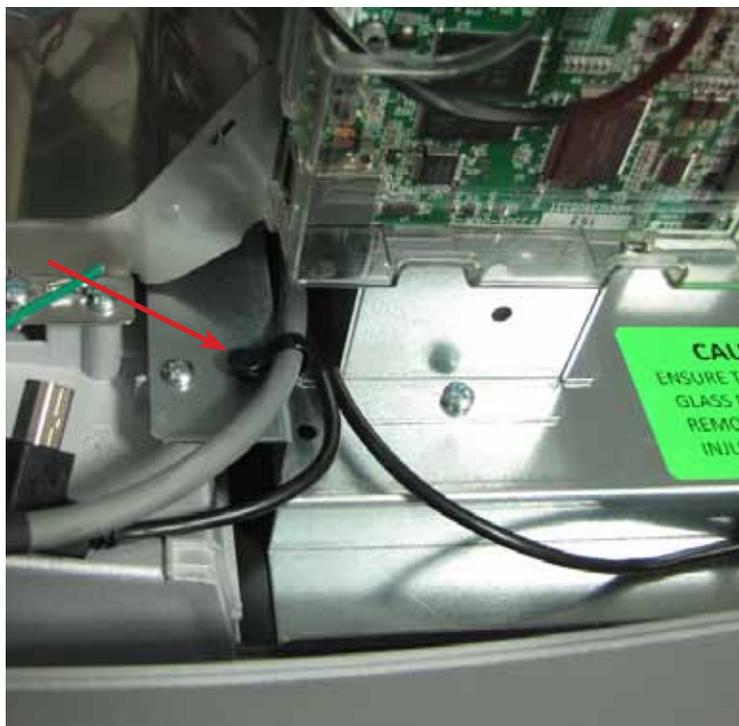
10. Install the new printer presenter support bracket with the 2 self tapping screws.
