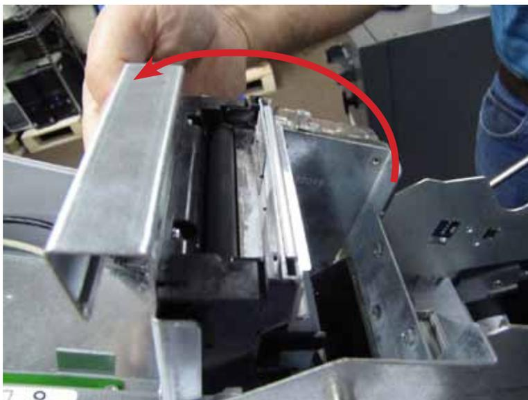
4. Remove the printer by removing the 4 screws holding it in place. Retain the screws for step 11.
