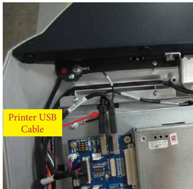
9. Remove the cable clamp holding the printer cable to allow room to install it on the new printer assembly.
