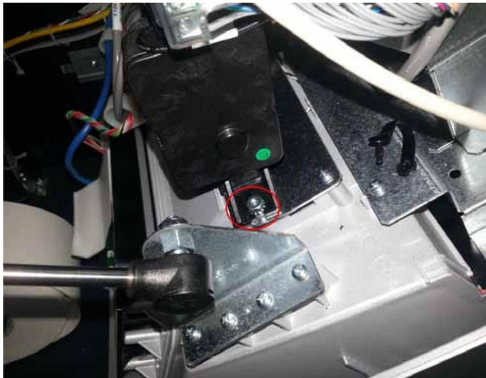
14. Plug the printer cable into the printer board. Connect the printer cable ground wire as shown. Route the USB cable as shown and plug into the board. Secure the printer cable and the USB cable with cable clamp and screw provided in the kit.
