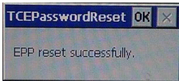
29. If Resets are complete, press 3 on the USB keyboard to select “Exit” from the main menu. ATM will restart. Remove the USB drive or Compact Flash Card.
