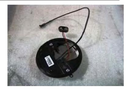
Connect the 9 volt battery and place inside the lock dial.
