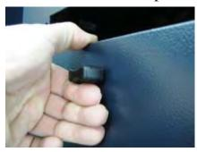
Apply Lock-Tite to the two shoulder screws. Install the two screws into the door as shown.
