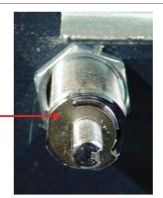
6. Install the latch cam, lock washer (retained from disassembly), and nut.
