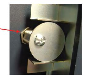
4. Position the new lock as shown (locked) and insert into the door. Hold the lock assembly as shown to ensure the tumbler mechanism does not come out throughout the rest of the installation. Secure the lock with the nut provided.
