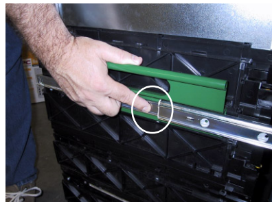
Figure 3. Push in on the mechanical stops (on both sides of the dispenser) to allow the dispenser to be pulled off the rails. Use 2-person lift!
