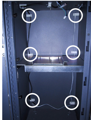
Figure 1a. Ensure power and phone cords are routed through cable clips. (TDM-100/MiniMech cabinet)
