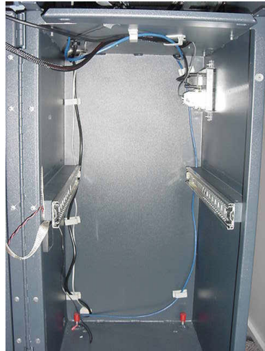
Figure 1b. Ensure power and phone cords are routed through cable clips. (SDD/NMD-50 cabinet)
