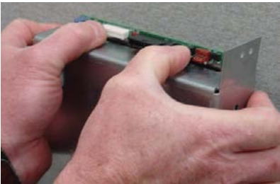
Figure 2-23a. Housing separation. Avoid contrast adjust!
