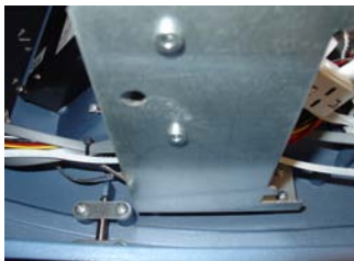
Figure 14. Route ribbon cable under Docking board bracket.
