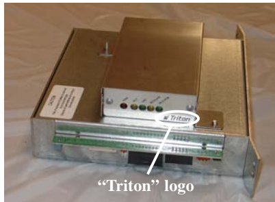
Figure 2-32. Install Ethernet assembly and bracket to mounting screws.
