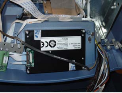
Figure 18. Reconnect ground harness.
