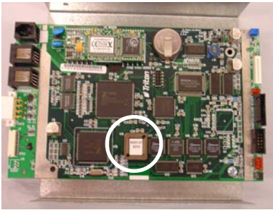
Figure 5. Eprom chip location.
