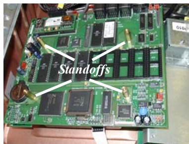
Figure 15. Main board secured.
