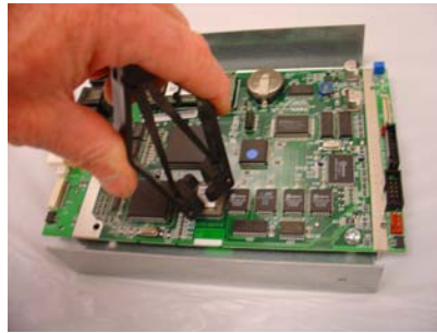
Figure 6. Remove Eprom chip.
