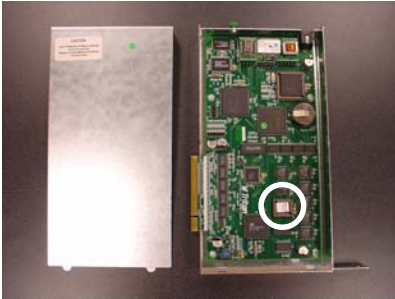
Figure 5. Eprom chip location.
