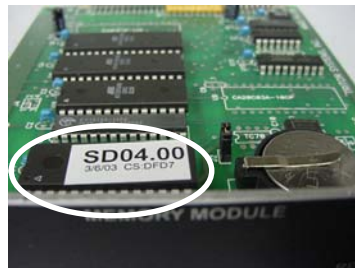
Figure 2-13. Memory module EPROM location.
