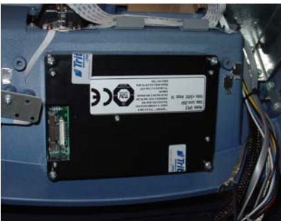
Figure 12. Install the EPP.
