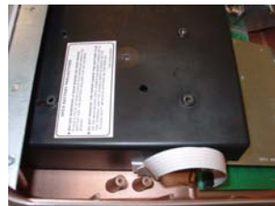
Figure 17. Connect/secure function key cable.
