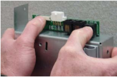
Figure 3. Housing separation. Avoid contrast adjust!
