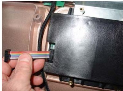
Figure 5. Connect adapter cable to EPP.
