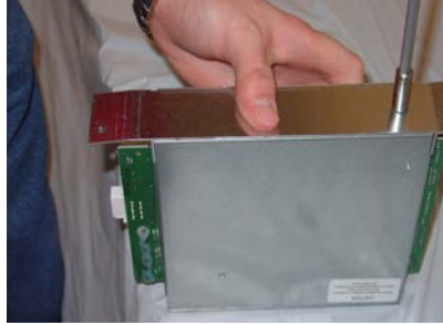
Figure 2-22b. Bottom screw location.
