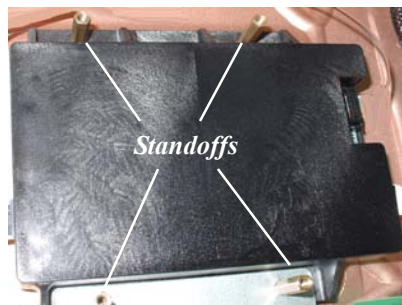
Figure 10. Secure with standoffs.
