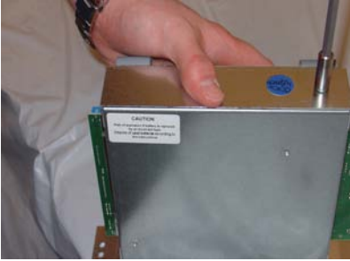
Figure 2-22a. Top screw location.
