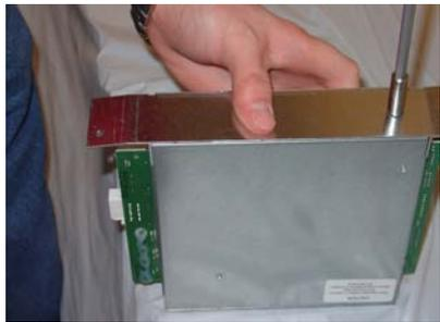
4. The following steps involve separating the Main board housing. The housing for the Main board is actually two (2) panels that fit together.
