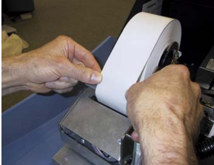
Figure 5-5. Feed paper into the printer take-up slot.
