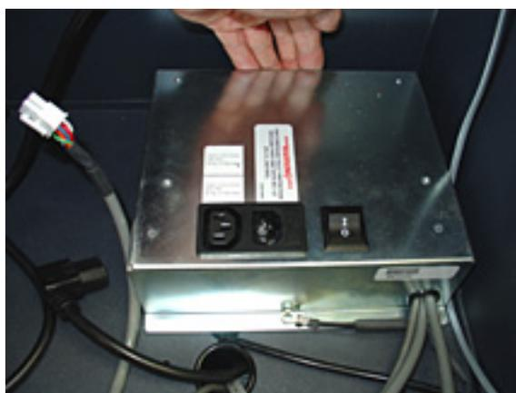
Figure 7. Removal of the single power supply from the cabinet top enclosure
