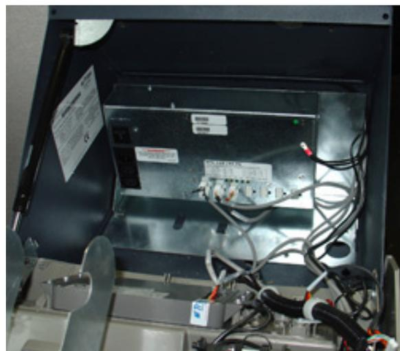
Figure 26. Slack in cabling tucked behind the power supply adaptor bracket
