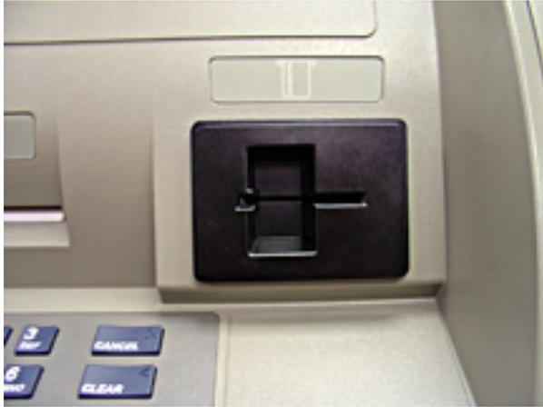
Figure 15. EMV card reader orientation as viewed from the front of the 9100 X2 control panel
