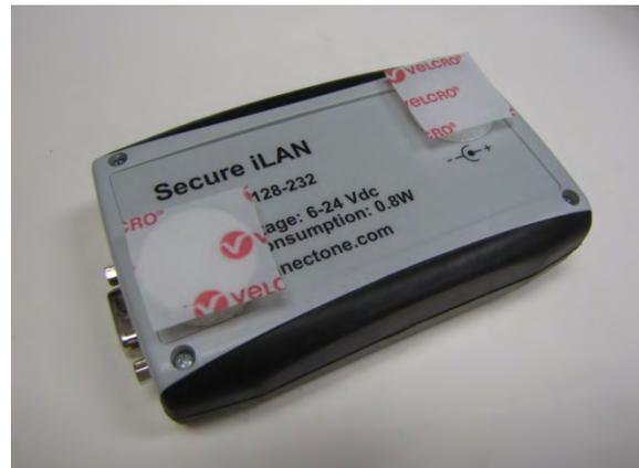
**Step 3:** Remove the paper backing from the hard pieces of Velcro. Place the iLAN box into the bracket with the serial port facing the side of the bracket with the metal lip as shown below. The iLAN box should be positioned against the bracket lip with extra bracket on the Ethernet port side. Once in place, gently push the box against the bracket to adhere the sticky side of the hard Velcro pieces.
