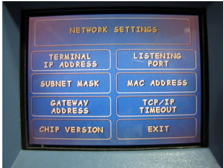
**Step 13:** Select “Change” to enter the “Terminal IP Address”. Using the keypad, enter the Terminal IP Address. (To enter a dot character, press the “Blank” key then press the “0” key TWICE to select the dot. Press the RIGHT ARROW key to lock it in.) Select “Exit” to save changes and return to the “Network Settings” page.
