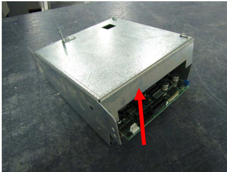
**Step 6:** Using side cutters, cut the TY Wrap that secures the modem module. Discard the TY Wrap. Remove the modem module by gently lifting it straight up unseating it from socket.
