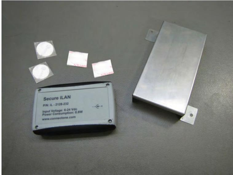
**Step 2:** Peel the paper backing off the two soft pieces of Velcro. Adhere them to the iLAN box as shown. Once the soft Velcro is secured in place, Velcro the hard sides to the soft pieces as shown.
