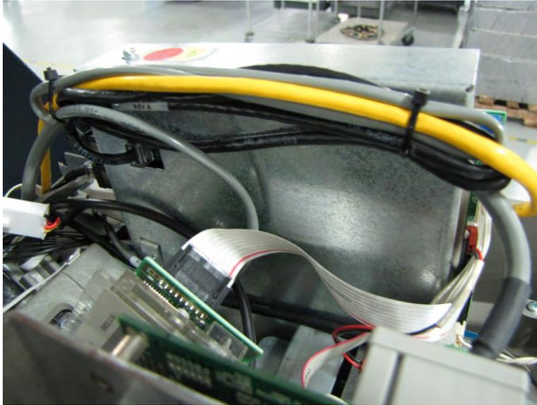
**Step 14: (Shallow cabinet)** Route the Ethernet cable through the cable clip and down through the middle opening and into the lower cabinet as shown below.
