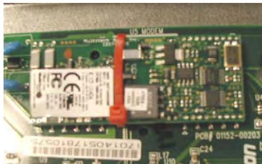
**Step 7:** The two screws securing the main board need to be replaced. Remove the screw holding the TY Wrap clip and replace it with the #8-32 – 1" Flat Headed Phillips screw. Ensure the TY Wrap clip remains on the board. Remove the second screw and replace it with the #8-32 – 3/4" Pan Headed Phillips screw. The screws will protrude on the backside of the cover.
