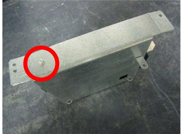
**Step 5:** Gently separate the top and bottom of the main board cover. Set the top aside.
