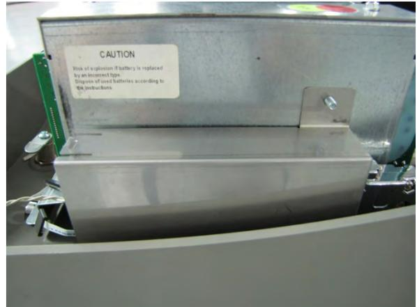
**Step 7:** Secure the bracket to the posts with the two #8-32 Hex Nuts.
