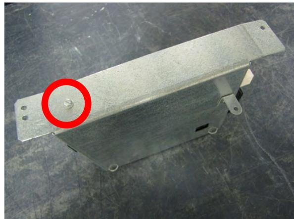
**Step 10:** Reinstall the main board assembly into the unit with the three screws removed in Step 3.
