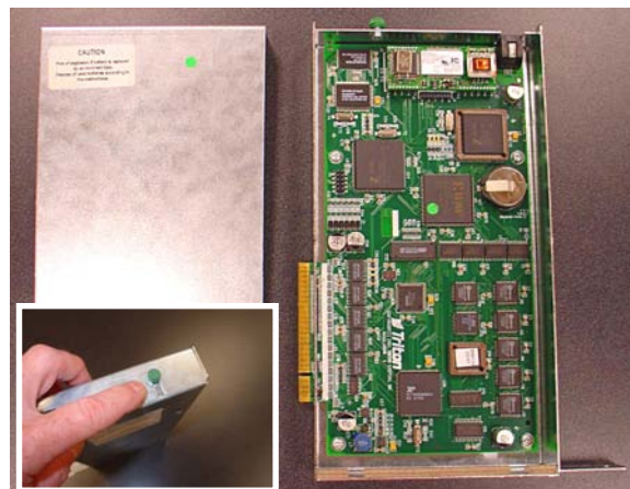
Figure 4. Main board assembly separated.
