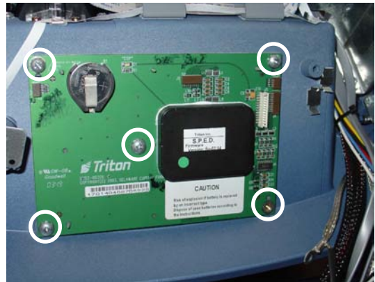
Figure 11. Remove screws and SPED board assy.
