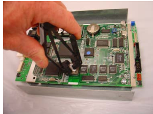
Figure 6. Remove Eprom chip.
