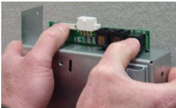
Figure 3. Housing separation. Avoid contrast adjust!
