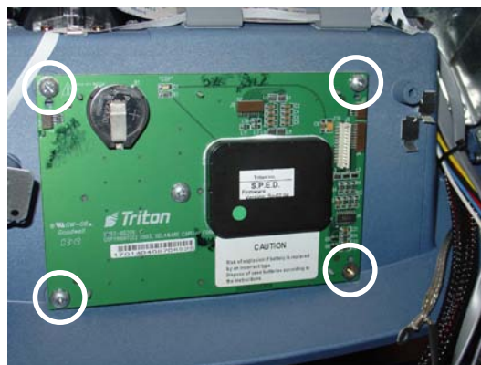
Figure 9. Remove SPED screws.
