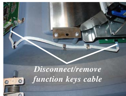
Figure 8. Disconnect/remove ribbon cable.
