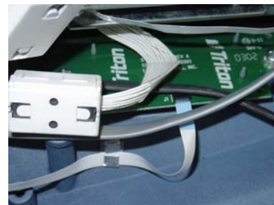
Figure 15. Left function keys circuit board.
