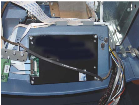
Figure 18. Reconnect ground harness.
