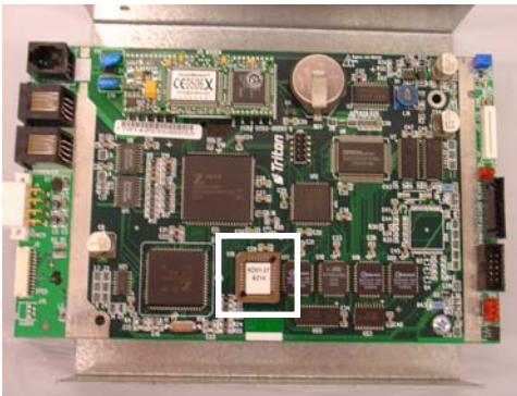
Figure 5. Eprom chip location.
