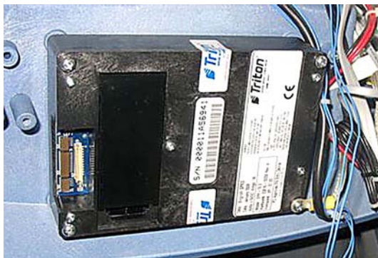
Figure 12. Install the EPP.
