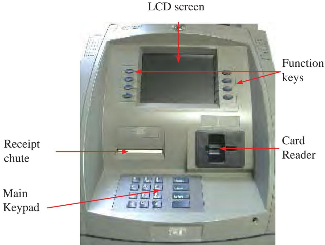
Figure 2-1. Control panel layout.
