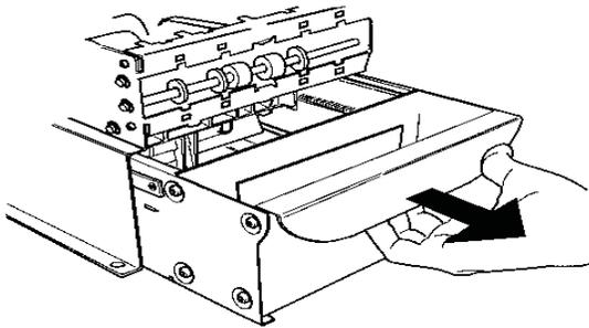
*Removing note tray from the dispensing mechanism.*
