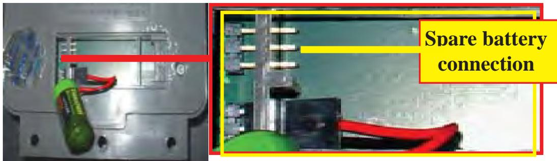
**EXISTING BATTERY - DO NOT REMOVE BEFORE CONNECTING A SPARE BATTERY FIRST!**
