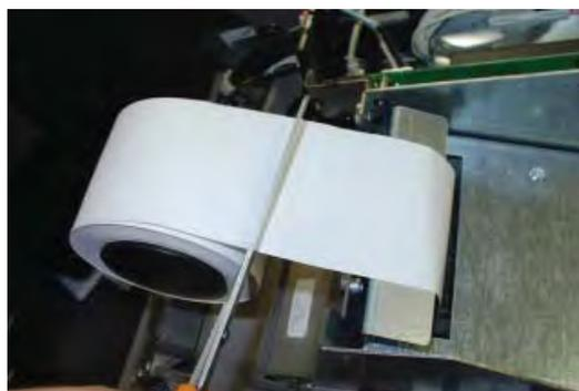
*Cut paper between the roll and printer feed path.*
