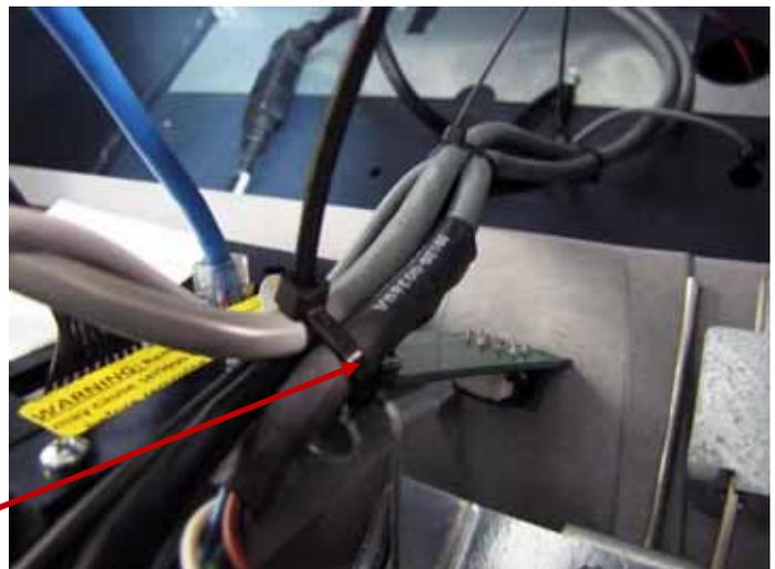
**Note:** The headphone pc-board mounting bracket has a cable routing feature built-in to secure a zip-tie.
