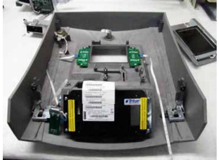
**9.4**—Partially route the flat cables under the clips on the new control panel as shown. Close the clips by folding down on the tabs.
