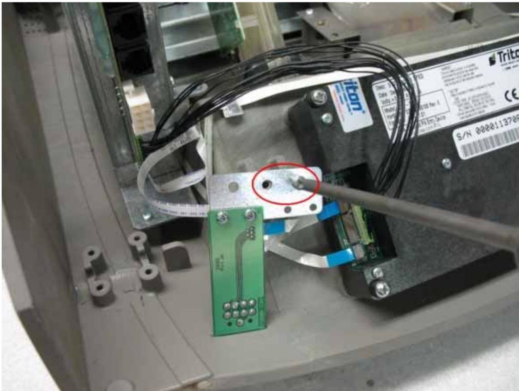
4.5—Remove the headphone board/bracket/cable from the old control panel.
