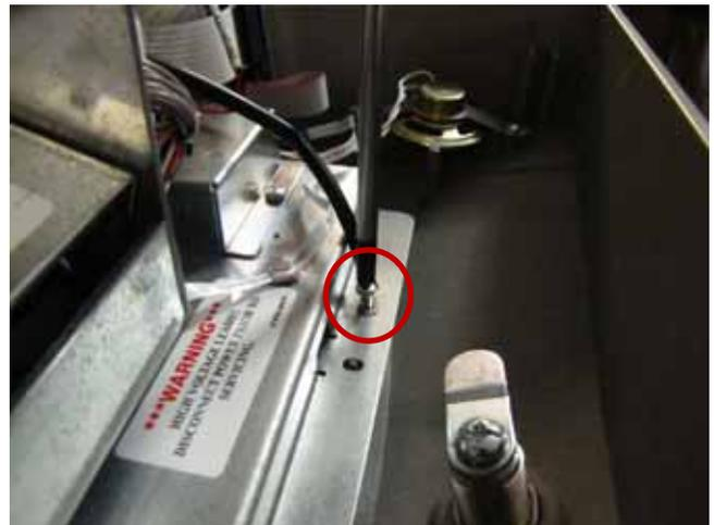
**1.3**—Cut the zip ties that hold the cables together. Unplug the power cables, telephone cable, SPED cable, and EJ/dispenser cable from the main board. (Note that there are more zip ties holding cables than shown in this photo.)
