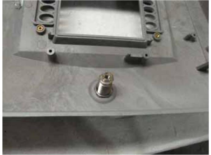
**2.4**—Place the lock pawl in locked position onto the lock body (See below for reference). Insert the retainer screw that previously held the lock cam in place and tighten. Use a torque between 22-30 in. lbs for the electric screwdriver
