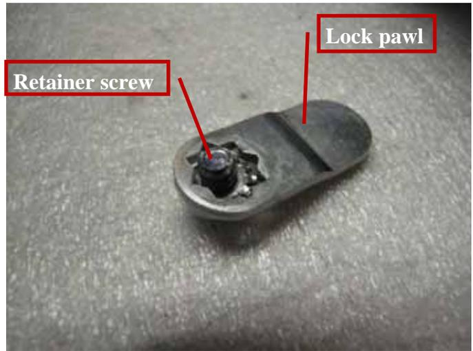
2.2—Note that the small tab on the top of the lock assembly should be facing the top of the panel. Remove the large nut with a 7/8" deep socket. Remove the lock and carefully keep it in the same position as before.
