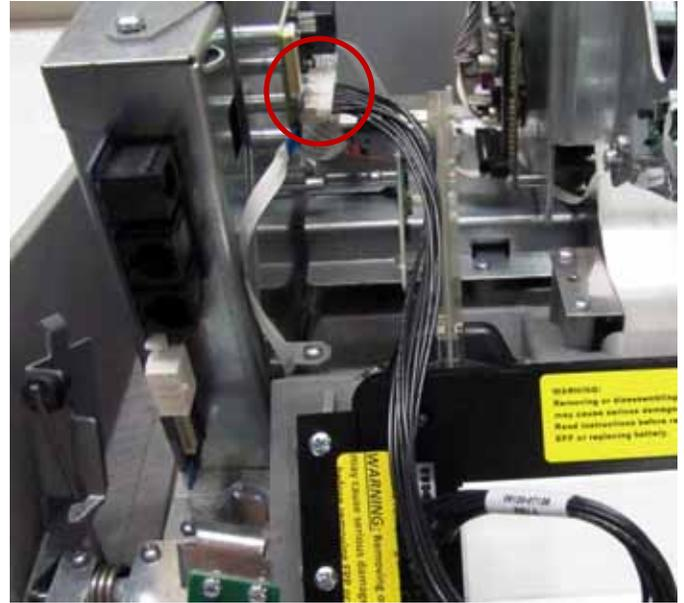
18.2—Plug the T9 EPP communications cable into the EPP and the T9 translator board connector.
