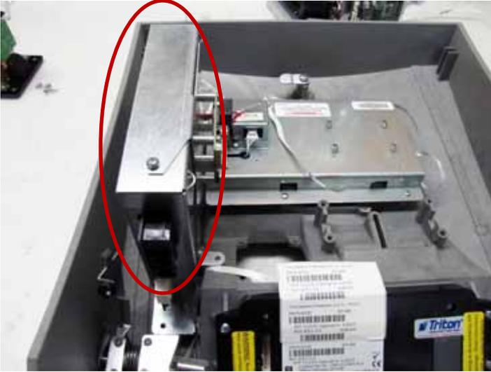
14.2—Install 3 screws to mount the main board housing.
