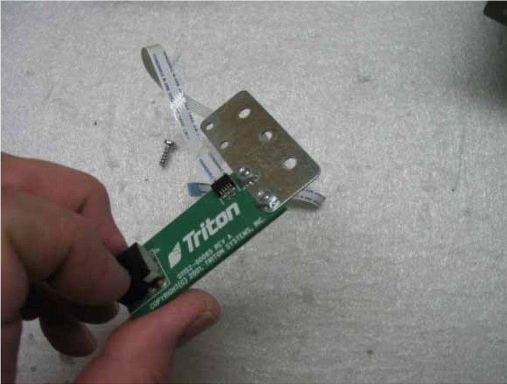
4.6—Remove the two screws and two nuts that hold the headphone board to the bracket using 1/4" nut driver and #1 screwdriver. Save these two screws and two nuts for installation on the new control panel headphone board bracket. Discard old headphone board bracket.
