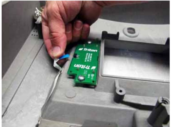
**9.2**—Remove the 2 screws from the left screen key board and install onto the new control panel. Repeat this process for the right screen.
