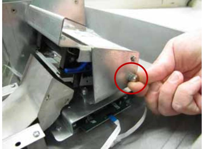
**16.4**—Route the low paper sensor cable under the sensor board and through the clip. Pinch the clips down to secure the cable. Plug the cable into the main pc-board.
