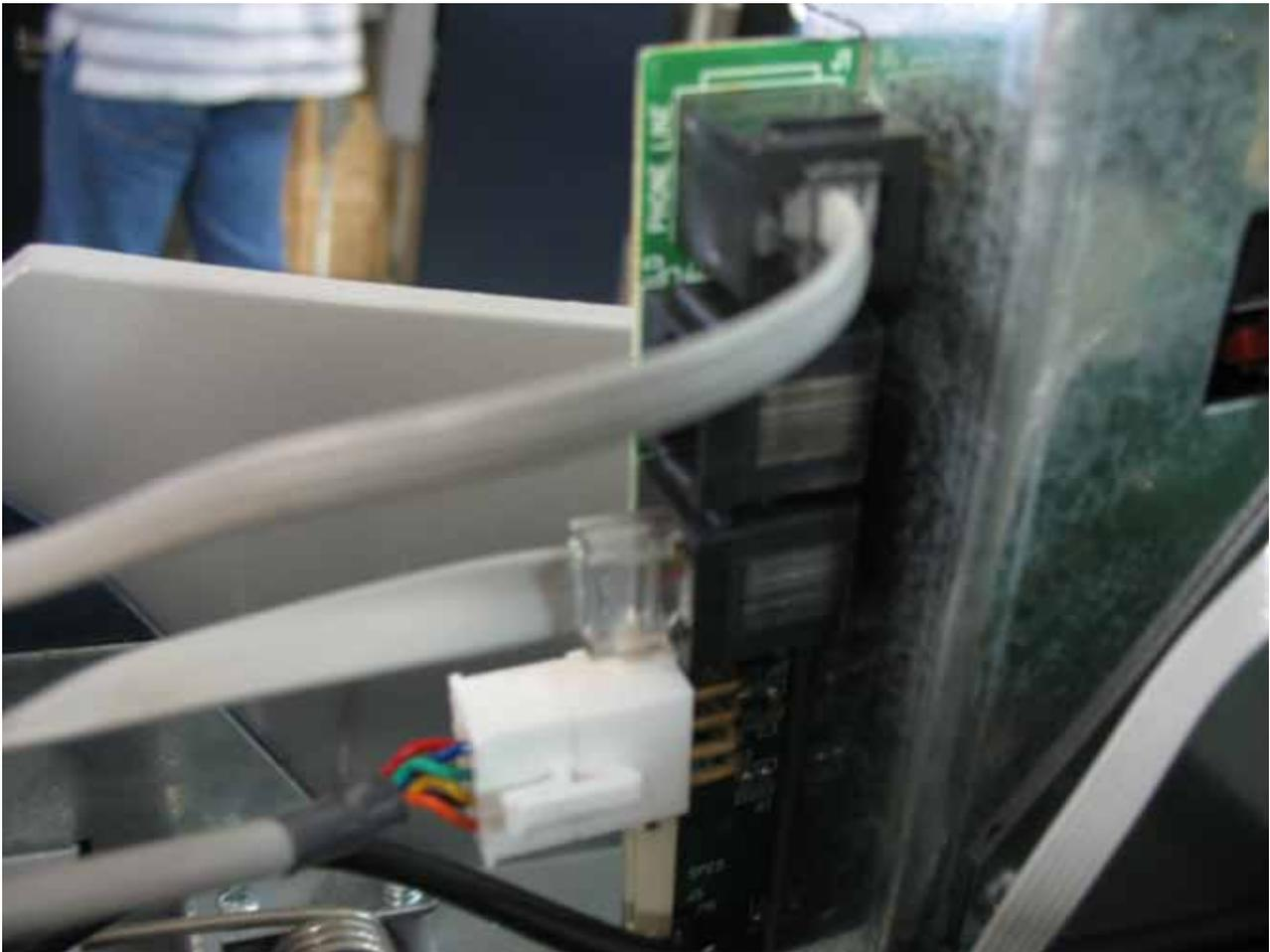
18.6—Secure all cables in place with proper length zip-ties.
