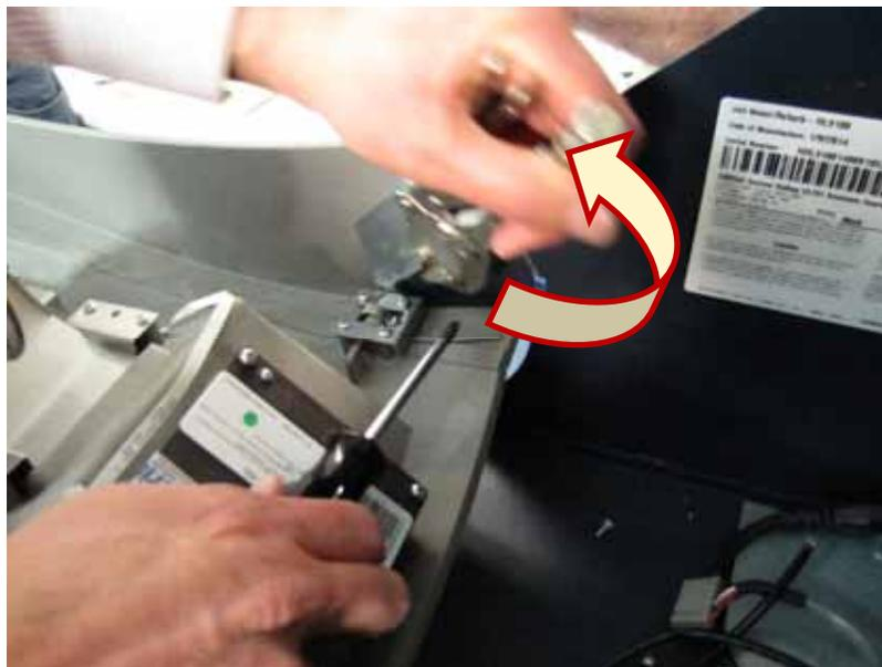
1.6—Remove the old control panel from the cabinet by partially closing the control panel until it's nearly in a vertical position, lifting, and pulling. Place the old control panel on a flat surface.
