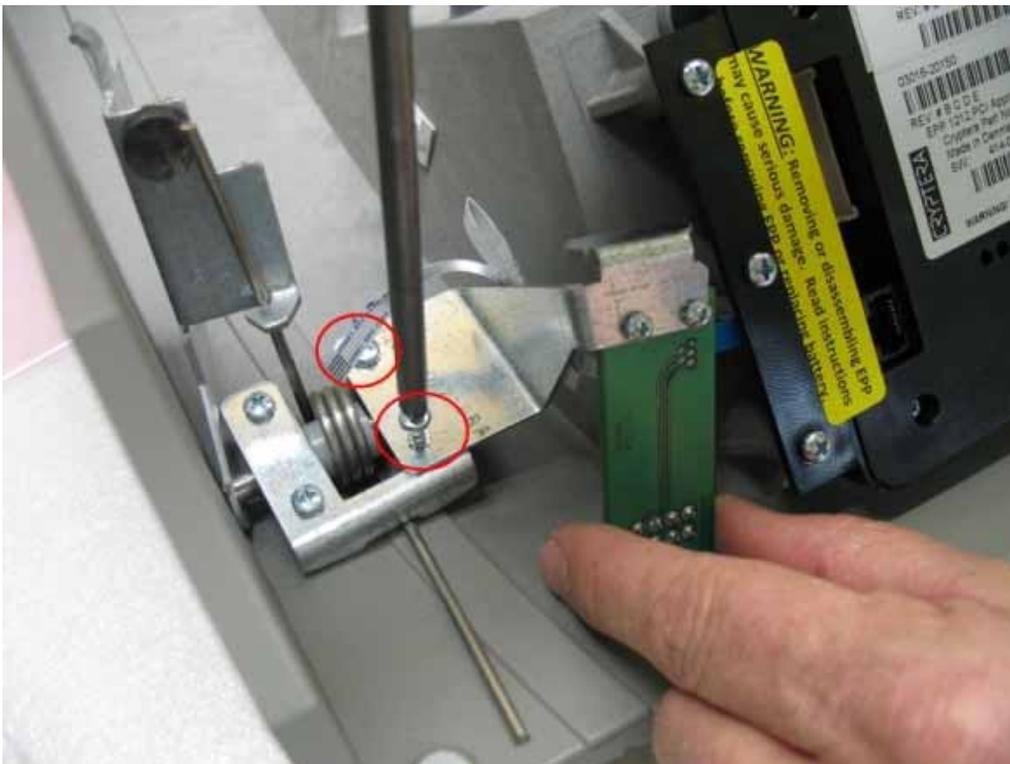
**4.12**—Loosen the screws that attach the headphone board to the bracket. Position the end of the headphone board snugly into the slot on the control panel and hold it down while hand tightening the headphone board screws.
