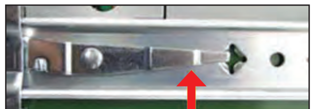
Figure 3 Slide rail, left side, push lever up to remove
