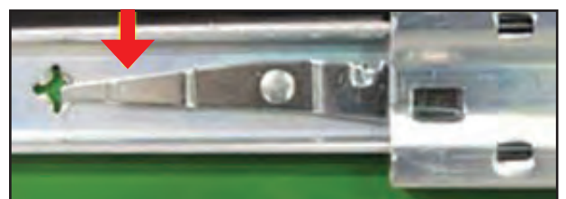
Figure 4 Slide rail, right side, push lever down to remove
