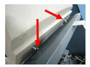
Step 13: Secure the midtopper to the cabinet with the four nuts previously removed in step #2.
