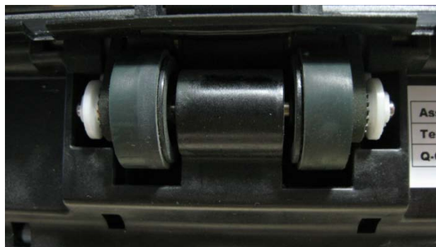
Smooth Rollers Used on NMD50 Revisions 1 and 2
