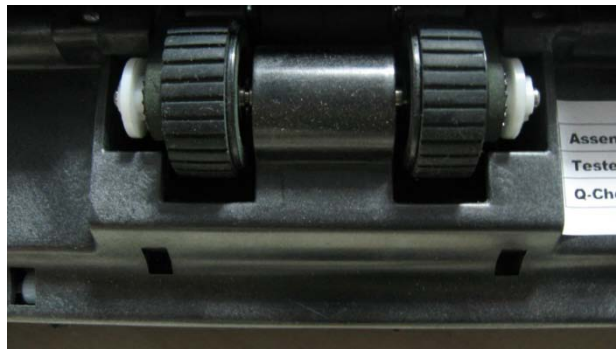
Tractor Rollers Necessary for Proper Polymer Note Picking
