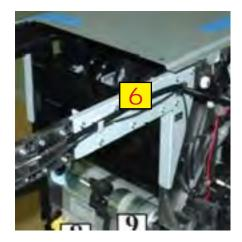
Additionally, remember to REMOVE and RETAIN the GREEN HANDRAILS before sending your NMD-100 dispenser to ATMGurus for T&M Repair. ATMGurus will not replace the green handrails. This new process is followed to reduce damage exposure during shipping of your repaired NMD.
