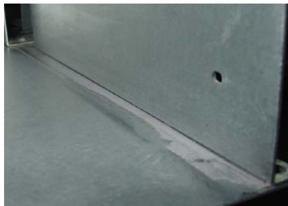
Peeling, worn Teflon strip
