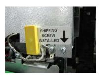
**Note:** Once the shipping screw is removed, it is recommended that it be retained for future use.
