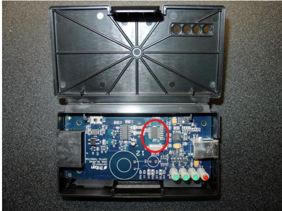
Location of the modem chip in the USB Modem (used in RL2000, RL5000, RT2000 and FT5000)
