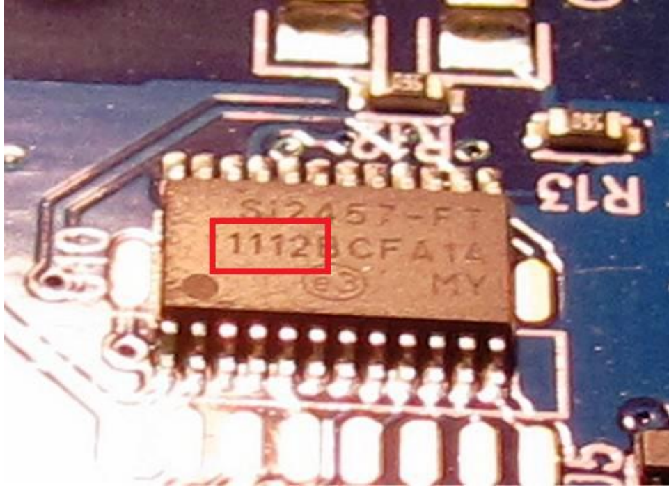
Modem chip showing date code from the defective lot (1112)
