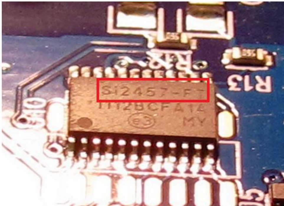
Location of the modem chip part number Si2457
