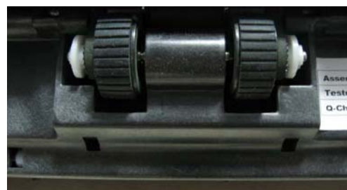
Tractor Rollers Necessary for Proper Polymer Note Picking
