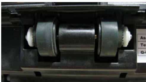
Smooth Rollers Used on NMD50 Rev 1&2
