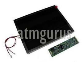
09110-20068 LCD Assembly, 8" Color, with LED backlight
