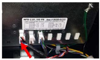
3. Plug the Power Adapter Cable into the Dispenser Power Cable.
