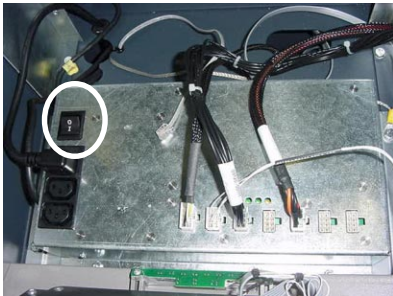
Figure 1. Power switch on left side of power module.
