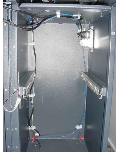
Figure 1. Ensure power and phone cords are routed through cable clips.
