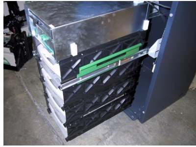
Figure 2. The NMD-50 dispensing mechanism fully extended on its mounting rails.
