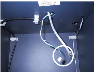
Figure 2. Dispenser data and power cables.
