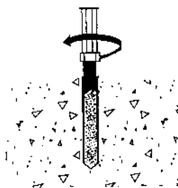
Fig. 6. Drive anchor rod into capsule using hammer drill.
