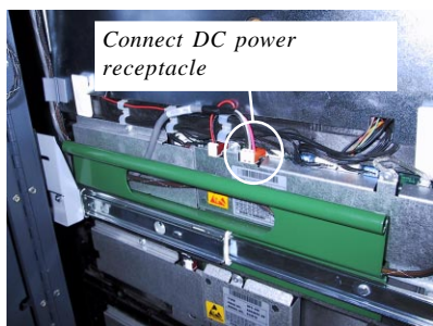
Figure 7. Connect the DC power plug to the receptacle shown above.
