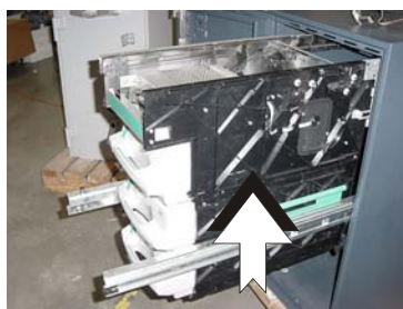
Figure 5. Lift dispenser off rails and guide out of cabinet. Use 2-person lift!
