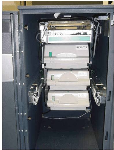
Figure 5. Slide dispenser into cabinet.
