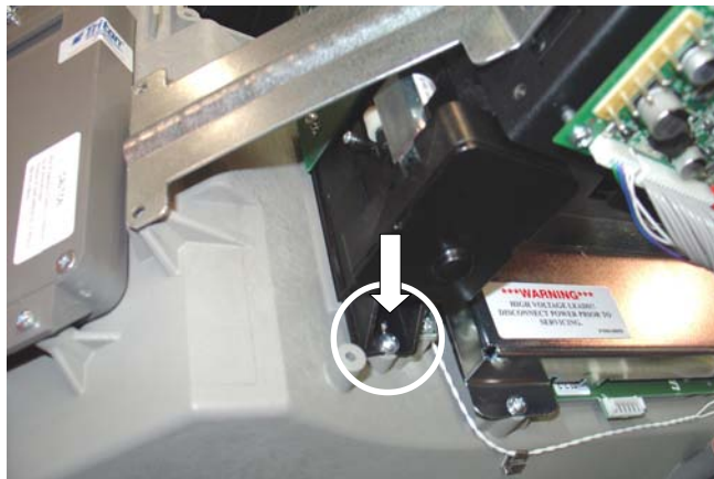
Figure 6. Start screw to hold assembly.
