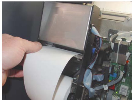
Figure 7. Insert receipt paper into printer.
