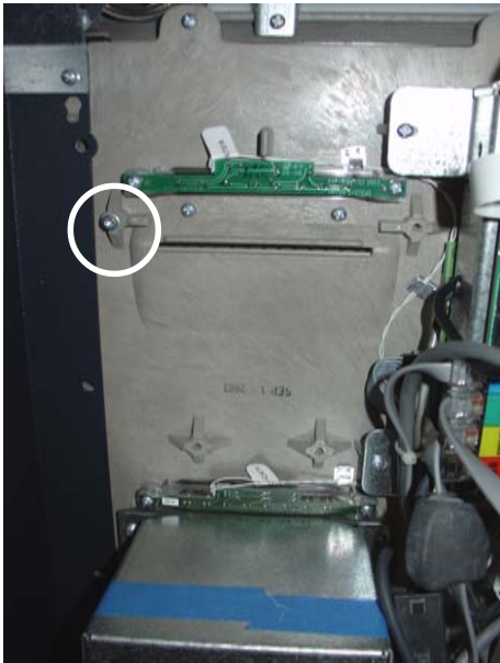
Figure 14. Start screw to hold assembly.
