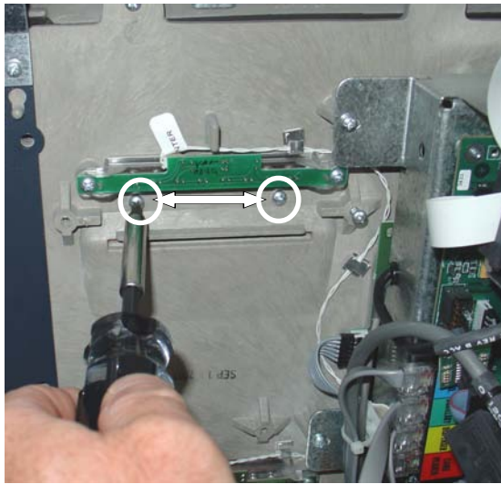
Figure 10. Remove 2 screws that secure bezel.
