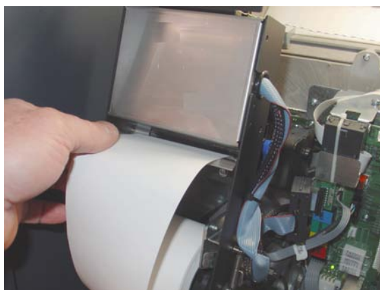
Figure 25. Insert receipt paper into printer.
