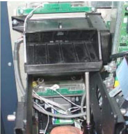
Figure 4. Remove Torx screws.
