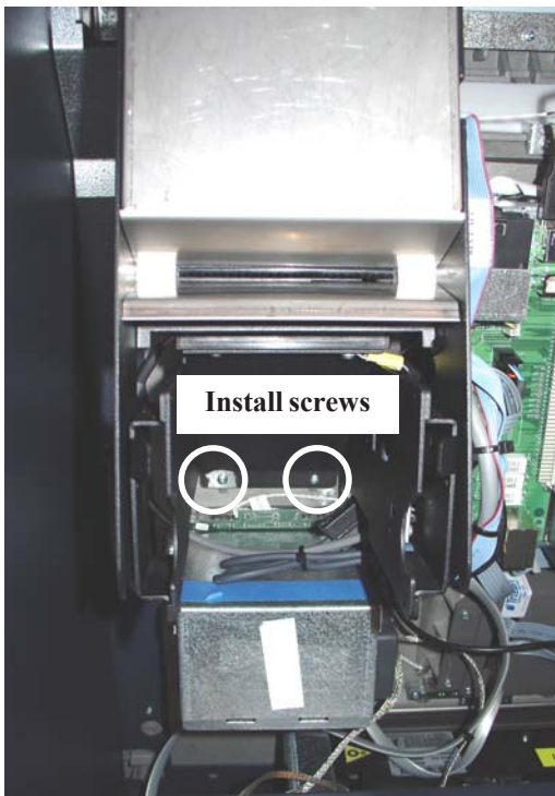
Figure 16. Printer mounting bracket secured.
