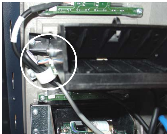
Figure 4. Disconnect presenter board cable.
