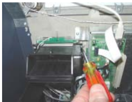
Figure 5. Remove phillips screws.
