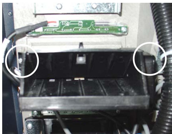
Figure 5. Remove screws and presenter assembly.
