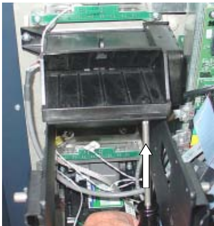
Remove Torx screws.
