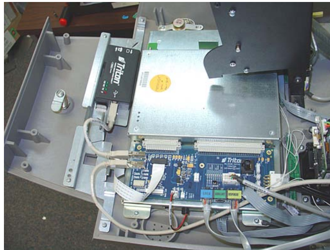
All cables routed/connected to Docking board.
