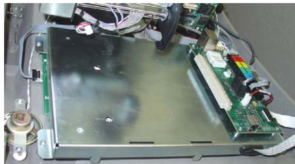
Main board removed.
