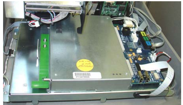
X2 main board installed.
