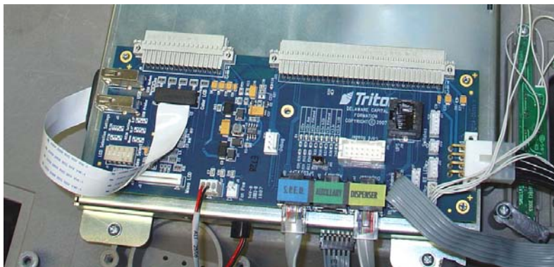
Docking board installed and some cables connected.
