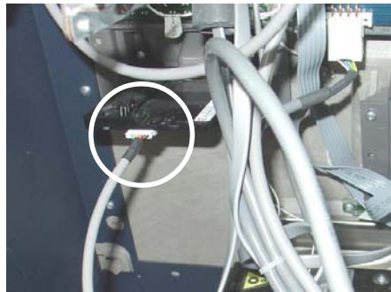
Remove/replace card reader cable.
