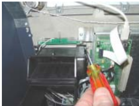
Remove phillips screws.
