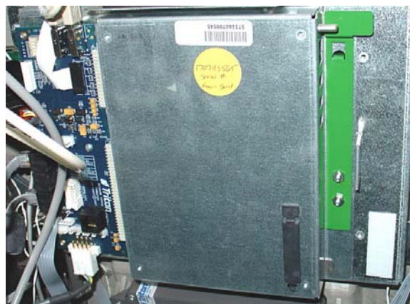
X2 main board installed.
