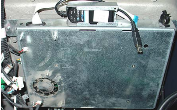
Docking board removed.
