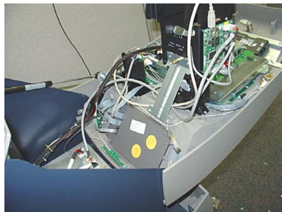
Route cables under strut.
