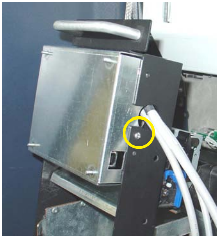
Insert cover assembly and secure right side with screw.
