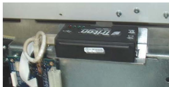
Mount/connect new modem.
