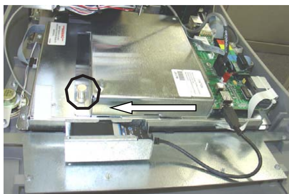
Pull release pin and slide assembly.
