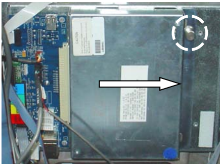
Pull release pin and slide assembly.
