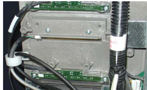
Presenter assembly removed.
