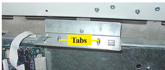
Install new modem bracket.
