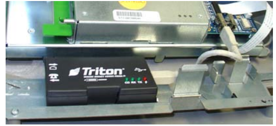
Mount/connect new modem.
