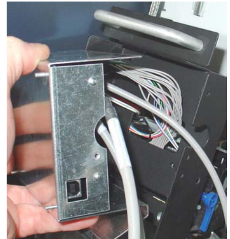
Face cover assembly towards printer bracket.
