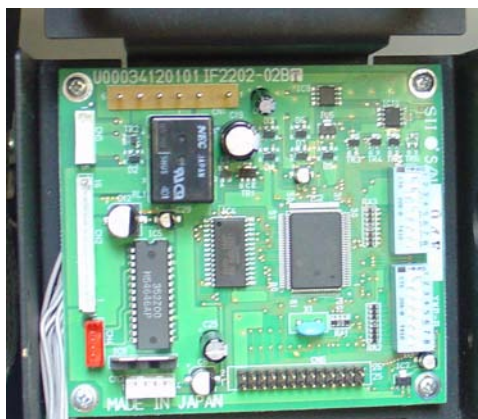
All cables removed from old controller board.
