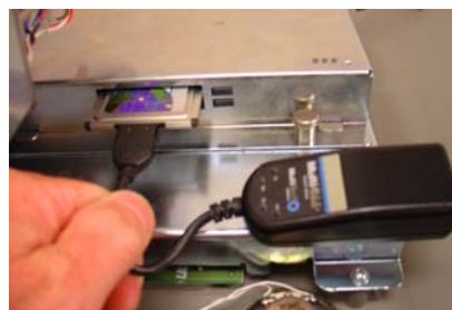
Remove PCMCIA modem card and phone line adapter.
