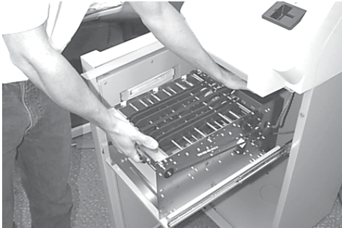
Figure 4. Installing the dispensing mechanism.
