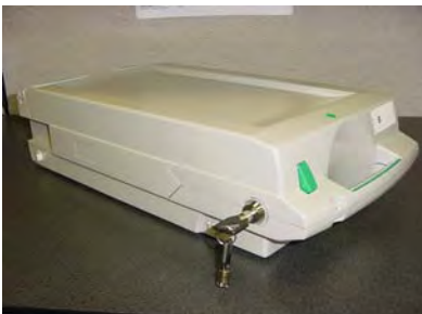
Insert key to unlock cassette.
