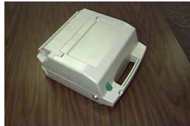
Reject cassette ready to open.
