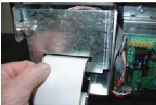
Figure 8. Paper feeds automatically in take-up slot.
