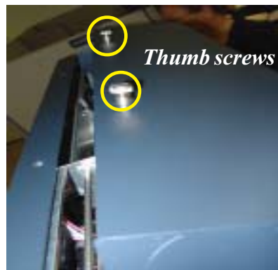
Figure 2. Loosen 2 thumb screws and remove back panel.
