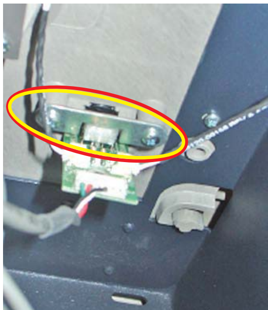
Connect speaker wires to audio board.
