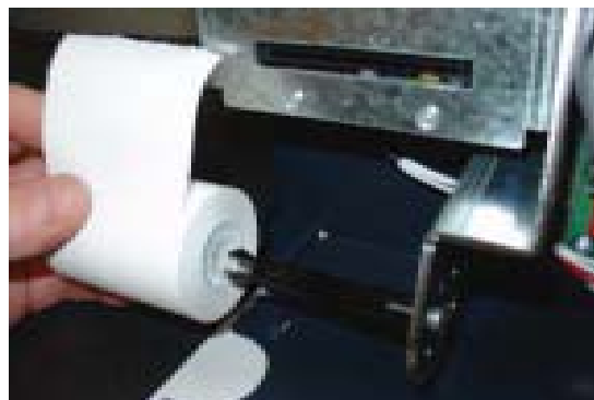
Figure 7. Insert paper roll on spindle (paper feeds from TOP ).
