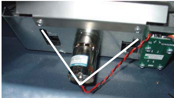
Screw locations for securing bottom of trim .
