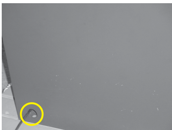
Left front side access hole.
