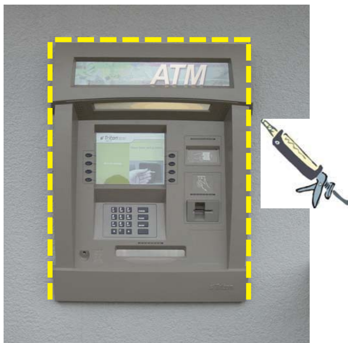
Control panel trim sealed.
