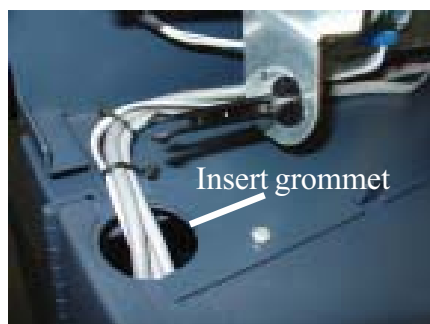
Figure 4. Feed cables through cable opening on top of cabinet.
