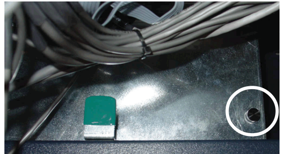
Remove retaining screw to open silver panel.
