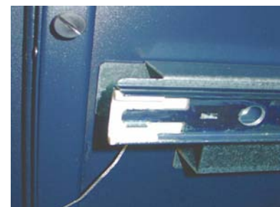
Figures 7 and 8. Slide rails flush w/bracket front.
