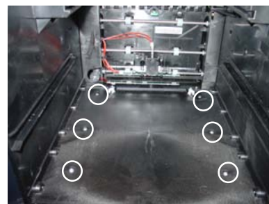
Figure 10. Remove mounting screws.
