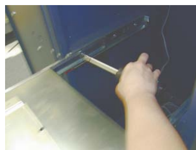
Figure 11. Remove slide rails w/tray.
