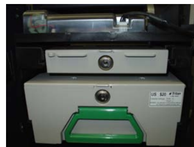
Figure 8. Mech in "Service" position.
