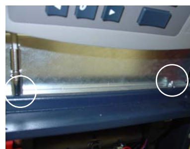
Figure 2. Loosen the 2 nuts that secure power supply.
