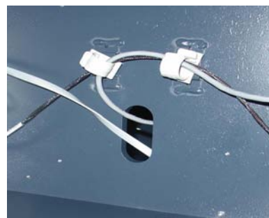
Figure 13. Route power/data cables.
