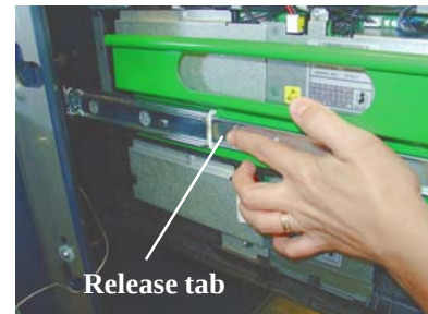
Figure 13. Push release tab.
