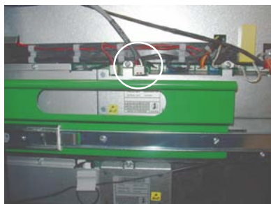
Figure 16. Power cable connection.
