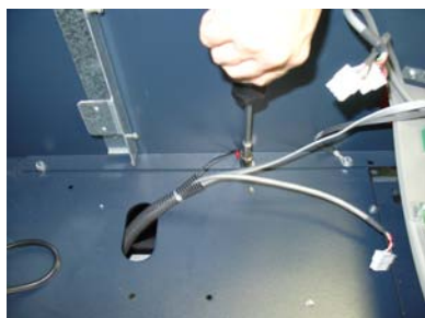
Figure 3. Disconnect ground wire.
