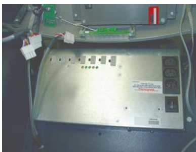
Figure 1. Disconnect all cables from power supply.
