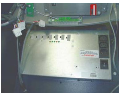
Figure 1. Disconnect all cables from power supply.
