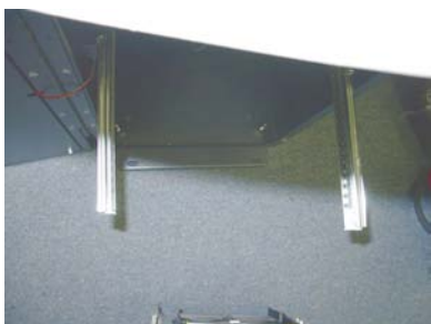
Figure 14. Rails extended (offset).
