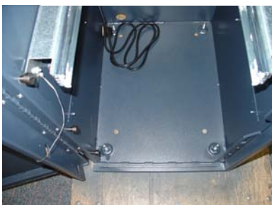
Figures 7 and 8. Slide rails flush w/bracket front.
