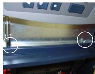
Figure 2. Loosen the 2 nuts that secure power supply.
