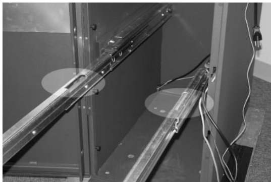
Figure 3-39. Mounting rails fully extended so that rail slots are visible.
