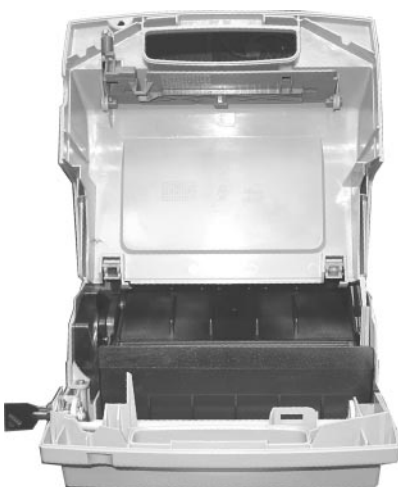
Figure 4-17. Reject Box open. Check both the single and bundle reject areas for rejected currency.
