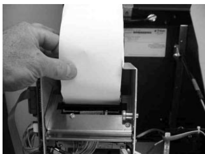
Figure 5-7. Feeding the paper into the printer.
