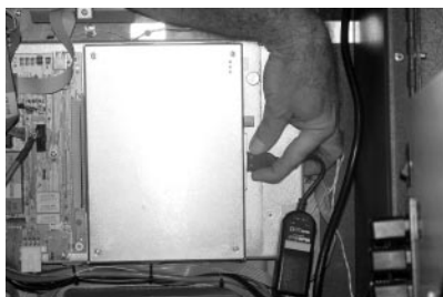
Figure 3-14. Disconnecting the telephone line adapter connector from the modem.
