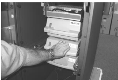
Figure 4-5. Installing a cassette into the NMD-100 dispensing mechanism.
