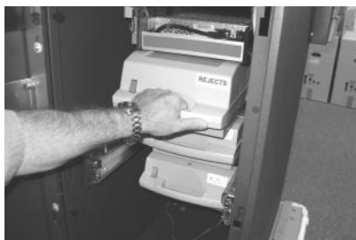
Figure 4-14. Remove the reject cassette by grasping the green handle and pulling it straight from the dispensing mechanism.
