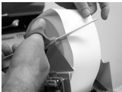
Figure 5-1. Cut paper between the roll and input to the printer.
