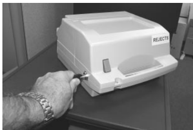
Figure 4-15. Unlock the cassette by inserting the key and turning it clockwise.
