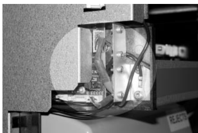
Figure 3-37. Unplug the serial communication and shutter cables .
