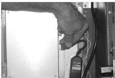
Figure 3-17. Connect the telephone line adapter connector to the modem.
