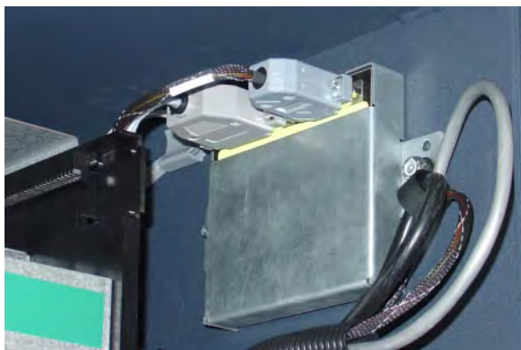
Figure 3-34. Electronic journal is installed in the upper right-hand corner of the Security Cabinet.
