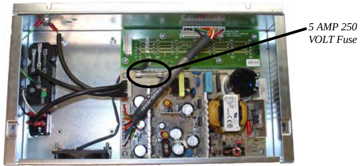
Figure 3-10. Remove the power supply from the cabinet to access the 5.0 AMP 250 VOLT fuse.
