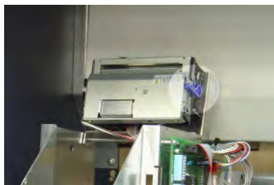
Figure 3-22. Rotate the blue lever down so it is perpendicular to the printer/cutter.
