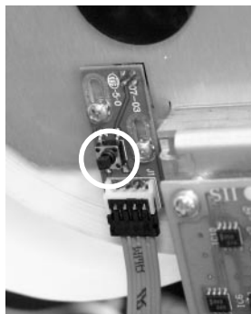
Figure 5-2. The paper feed button is located on the Paper Bracket.
