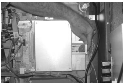
Figure 3-16. Installing the modem into the PC-MCIA slot.
