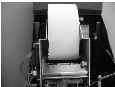
Figure 5-8. Paper roll and spool in place for operation.
