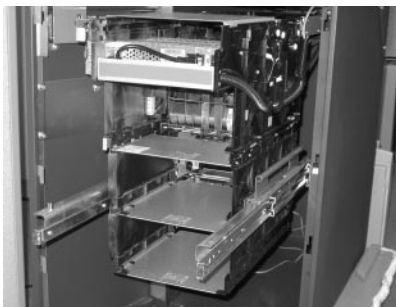
Figure 3-36. FT5000 dispenser extended with reject vault and cassettes removed
