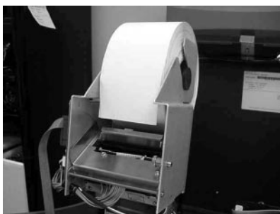
Figure 5-6. Paper on the paper support bracket ready to be loaded into the printer.
