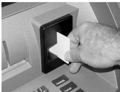
Figure 5-9. Use the cleaning cards on a monthly basis to maintain effective card reader operation.
