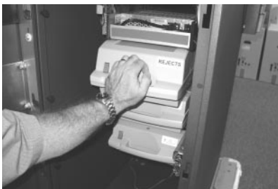
Figure 4-19. Installing the reject cassette.
