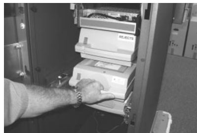
Figure 4-4. Removing a cassette from the NMD-100 dispensing mechanism.
