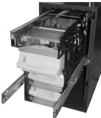
Figure 3-4. FT5000 Automated Teller Machine with cash dispensing mechanism fully extended from the cabinet.
