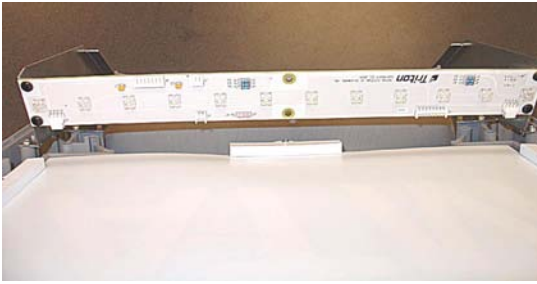
Lower LED installed.
