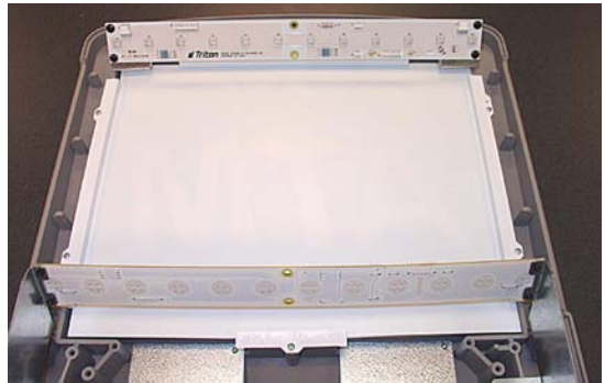
LED light bars installed.
