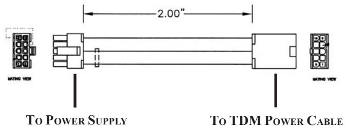
**Step 1: ENSURE POWER SWITCH IS OFF!** Disconnect all the cables (AC and DC) from the power supply.
