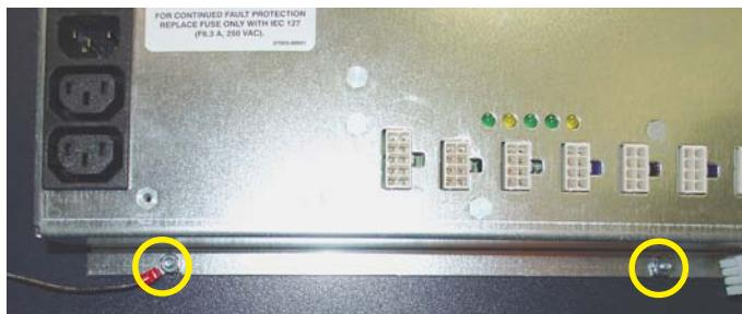
**Step 3:** Install the upgraded (dual) power supply provided following the steps in reverse. Reconnect all cables Except the TDM power cable
