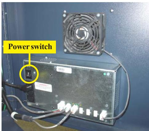
**Step 2:** Using an 11/32" nut driver, *loosen* the two (2) bottom nuts shown. Next, lift the power supply up and remove.
