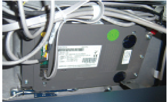
T5 PCI-EPP installed in the FT5000
