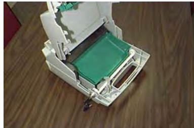
Figure 4-19. Bundle reject tray.
