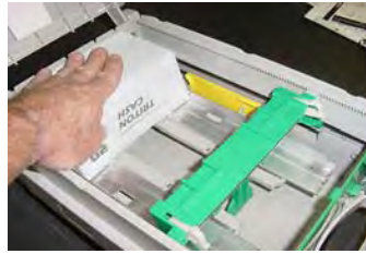
Figure 4-12. Leveling note pile.
