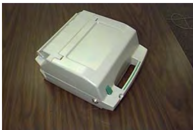
Figure 4-16b. Reject vault ready to open.
