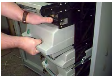
Figure 4-16a. Removing the reject vault.
