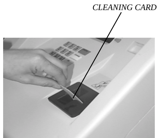
Figure 6-1. Use the cleaning cards on a monthly basis to maintain effective card reader operation.
