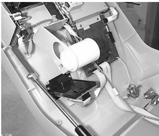
Figure 6-4A. Paper Spool in its normal operating position.
