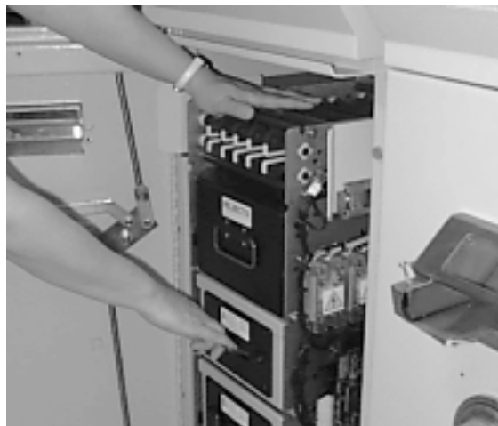
Figure 2-2. Removing a cassette from the dispensing mechanism.
