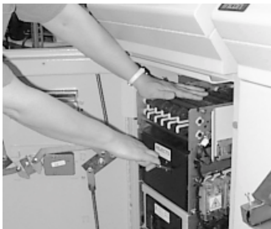
Figure 4-10. Removing the Reject Box
