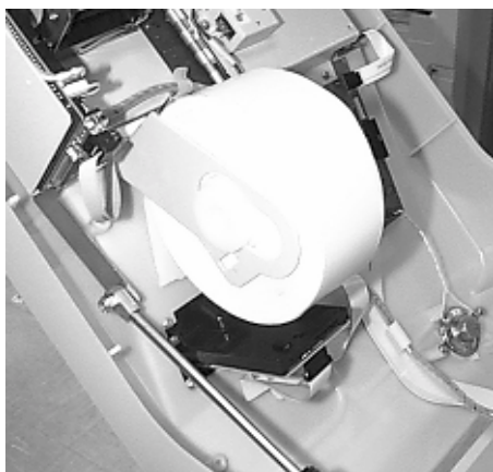
Figure 6-6A. Placing the paper roll and spool on the paper bracket.
