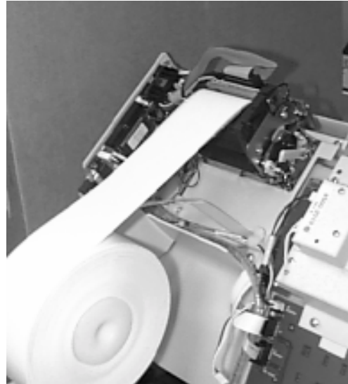
Figure 6-8. A new roll of paper installed on the Printer.
