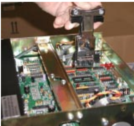
Figure 5. Remove old Eeprom from socket.
