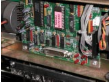
Figure 3. Locate original Eeprom chip.
