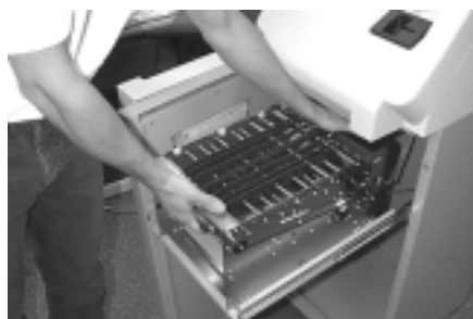
Figure 2. Lift mechanism from slide tray.
