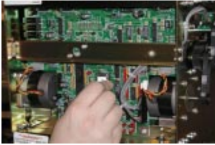
Figure 7. Align Eprom pins with socket holes.
