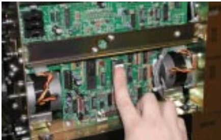
Figure 8. Press Eprom into socket.
