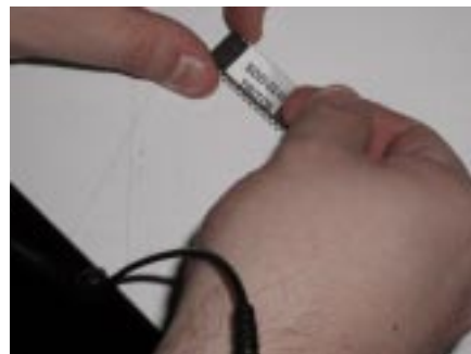
Figure 6. If necessary, bend pins on new Eeprom to help insertion.
