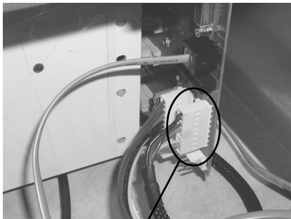
Step 17 - Re-connect Dispenser Power cable to J9 on backplane PCB.
