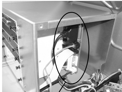
Step 3 - Disconnect all cables from the backplane board.
