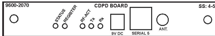
**Figure 3. CDPD Module Front Panel Features.**
