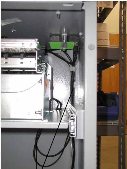
The cables should be routed through the back slide rail as shown.
