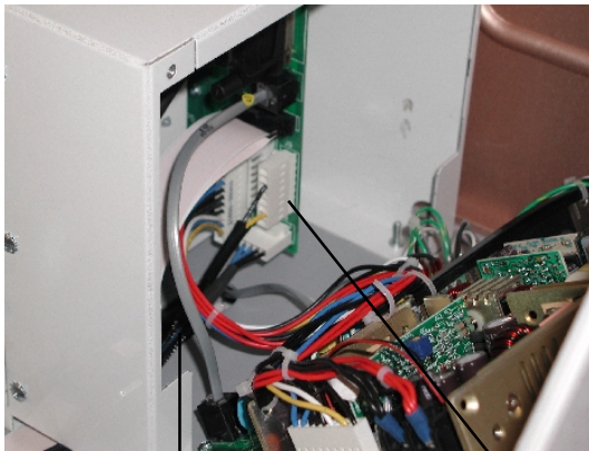
Route end of cable through hole in the cabinet
