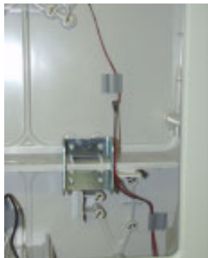
Figure 4-10. Fan Power Cable routed through two Hightopper cable clips.
