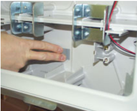
Figure 4-43. Secure 4-Pin Modular Cable in ATM Back Housing cable clip.
