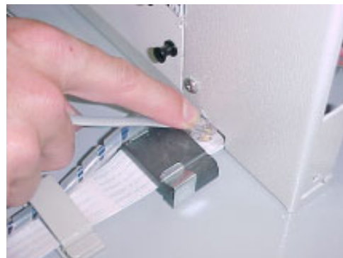
Figure 4-25. Inserting modular cable into Card Cage.
