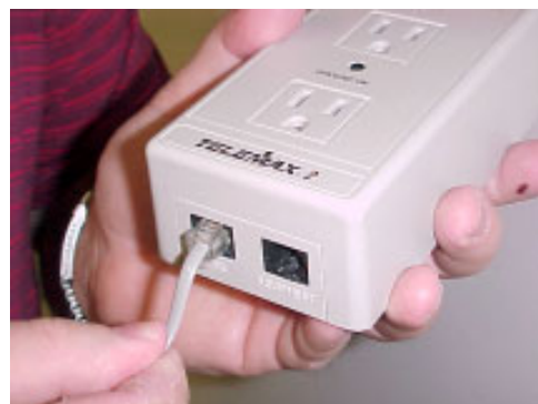
Figure 4-46. Connect modular patch cable to LINE jack.
