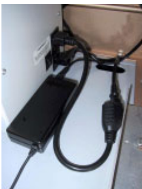
Figure 4-52. Connect module power cord plug to AC adapter cable.
