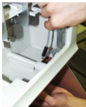
Figure 4-11. Feeding Fan Power Cable into ATM Upper Enclosure.
