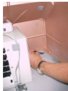
Figure 4-33. Feeding Line Sharing Device power cord into ATM upper enclosure.
