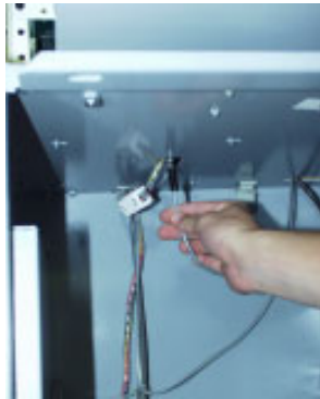
Figure 4-15. Feed Fan Power Cable into Card Cage.
