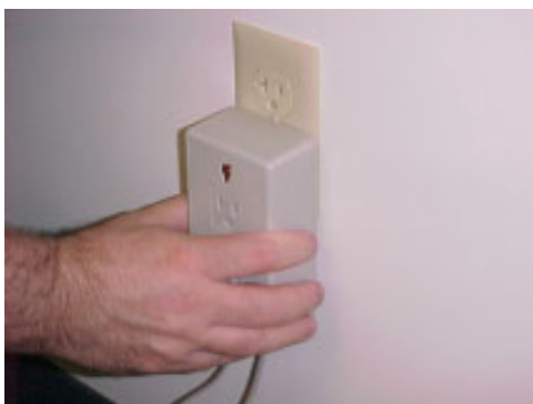
Figure 4-48. Connect Surge Suppressor to wall outlet.
