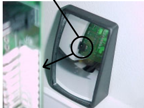
Figure 4-17. Mirror Shows FMV Fan Power Jack on Rear of Backplane.
