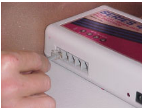
Figure 4-27. Connecting modular cable to LINE jack on Line Sharing Device.
