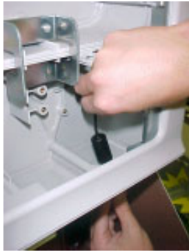
Figure 4-55. Pulling FMV Power Module cable into Hightopper.
