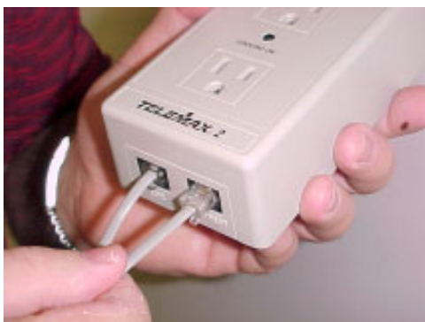
Figure 4-47. Connect Modular Cable to EQUIPMENT jack.
