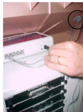
Figure 4-34. Connecting Line Sharing Device power cord plug.
