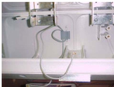
Figure 4-39. Connecting power cable connector to FMV.
