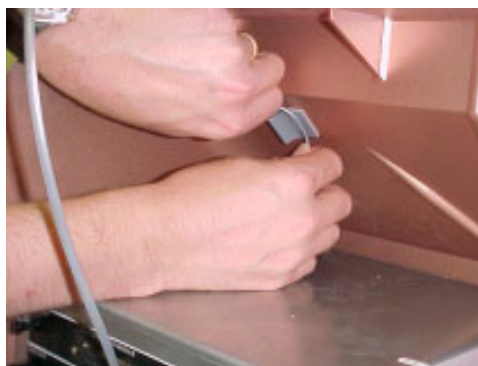
Figure 4-41. Secure 4-Pin Modular Cable in ATM back housing cable clip.
