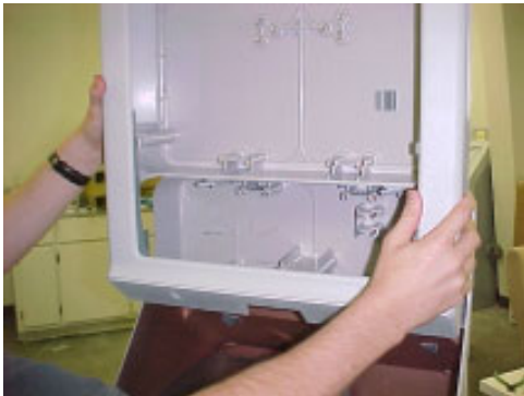
Figure 4-1. Place FMV Hightopper Housing on ATM.
