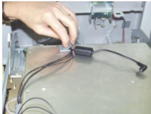
Figure 4-62. Routing power cable through FMV Hightopper cable clip.
