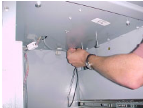
Figure 4-32. Feeding Line Sharing Device power cord into ATM upper enclosure.
