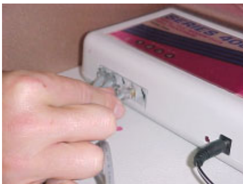
Figure 4-35. Connecting FMV modular cable connector into Line Sharing Device.
