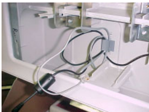
Figure 4-57. Secure FMV Power Module cable (and modular cable) in cable clip.
