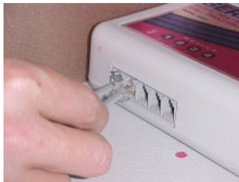
Figure 4-29. Connecting modular cable to DEVICE 1 jack on Line Sharing Device.
