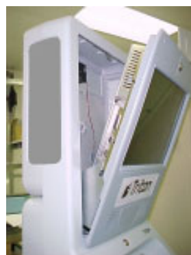
Figure 4-67. FMV Door Panel opened to normal access position.
