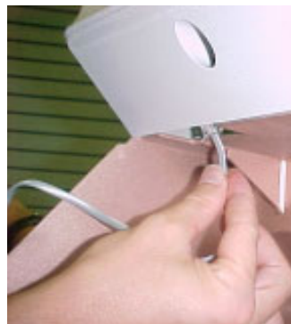
Figure 4-37. Connecting power cable connector to FMV.
