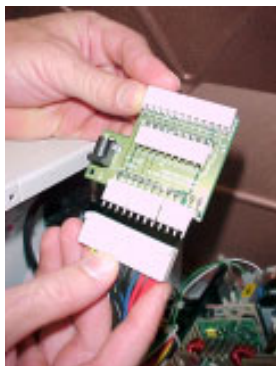
Figure 4-20. Connect Power Supply Cable to J1 on Adapter Board.
