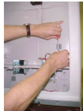
Figure 4-9. Routing Fan Power Cable through cable clip.
