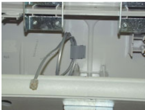
Figure 4-44. Secure 4-Pin Modular Cable in ATM Upper Enclosure cable clip.
