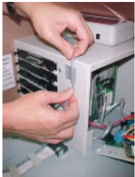
Figure 4-30. Routing modular cables through cable clip.
