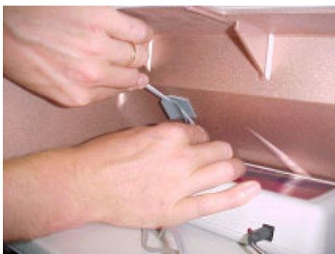
Figure 4-36. Connecting power cable connector to FMV.
