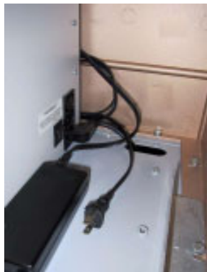
Figure 4-50. Place module power cord behind card cage.
