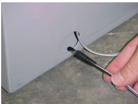
Figure 4-31. Feeding Line Sharing Device power cord into ATM.
