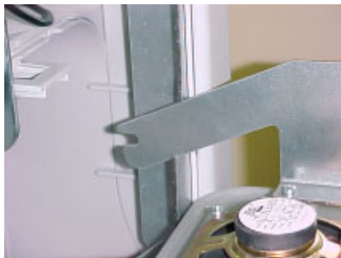
Figure 4-59. Closeup view of mounting bracket resting in notched support.
