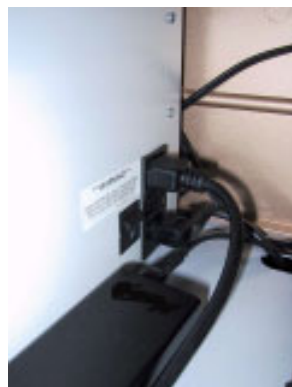
Figure 4-51. Connect AC adapter cable to card cage outlet.
