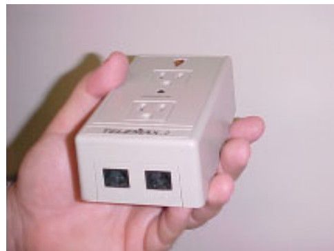
Figure 4-45. Note location of LINE jack (on the left).
