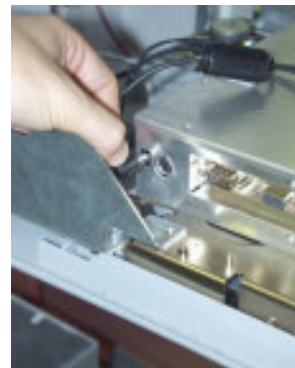
Figure 4-63. Connecting power cable connector to FMV.
