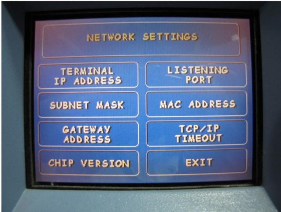
**Step 17:** Select “Change” to enter the “Gateway Address”. Using the keypad, enter the Gateway Address. (To enter a dot character, press the “Blank” key then press the “0” key TWICE to select the dot. Press the RIGHT ARROW key to lock it in.) Select “Exit” to save changes and return to the “Network Settings” page.
