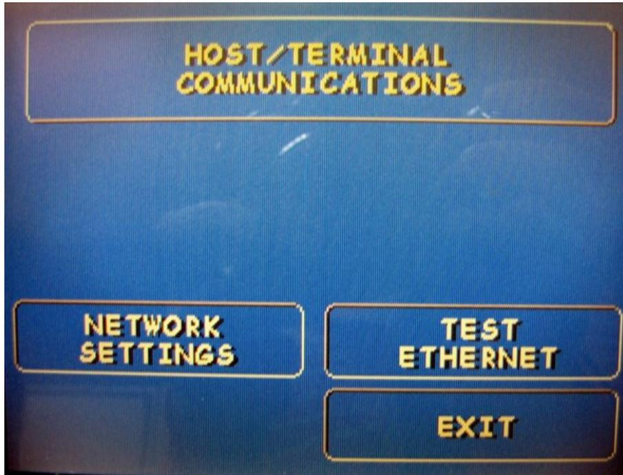
**Step 19:** The unit will test the Ethernet connection. Once you receive the “Tested OK” screen, press “CANCEL” on the keypad to continue. If you did not get an OK, retest the unit.
