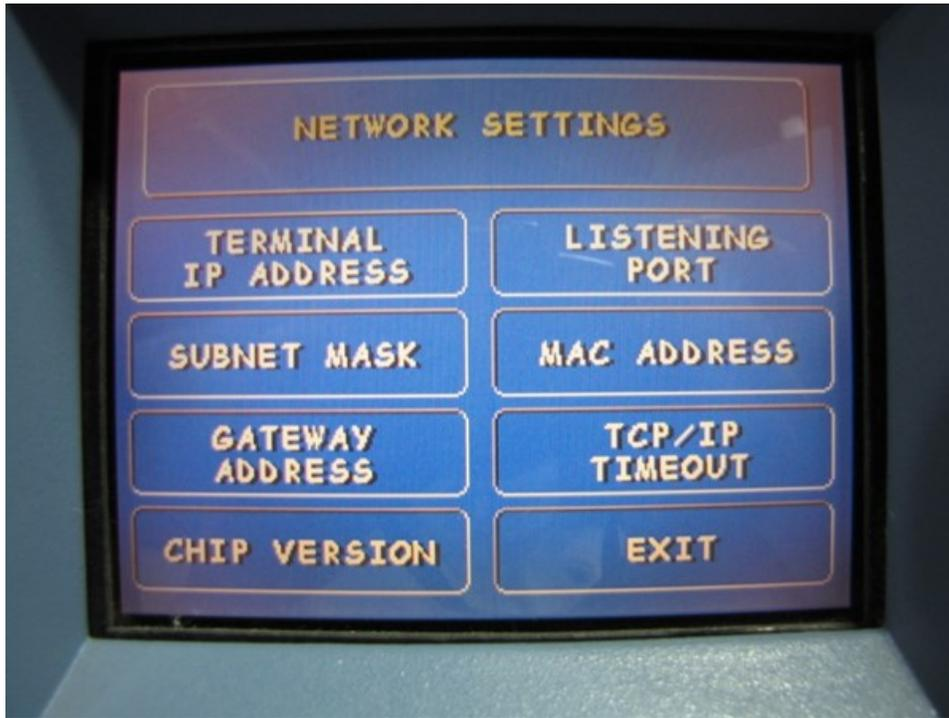
**Step 15:** Select “Change” to enter the “Subnet Mask”. Using the keypad, enter the Subnet Mask. (To enter a dot character, press the “Blank” key then press the “0” key TWICE to select the dot. Press the RIGHT ARROW key to lock it in.) Select “Exit” to save changes and return to the “Network Settings” page.
