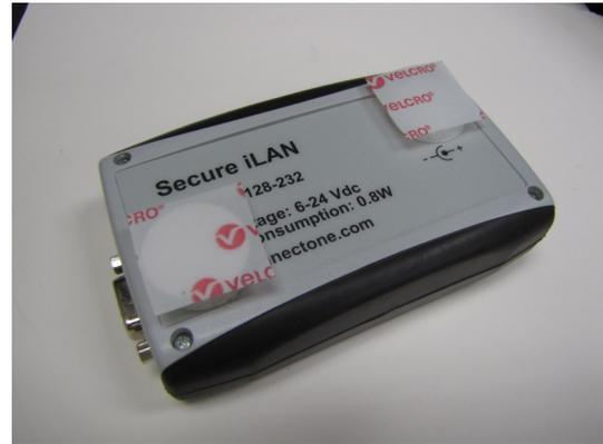
**Step 6:** Connect the Ethernet cable to the back of the iLAN External Ethernet box. Locate the communication cable. Connect the 9-Pin connector end to the back of the iLAN box (depending on connector end, you may need a small flat screwdriver to secure).
