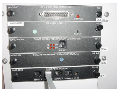
Figure 2-18. RJ-45 connected to Serial 2 of Quad Port module.
