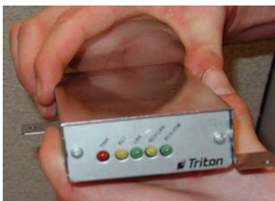
Figure 2-31. Mount external Ethernet bracket.
