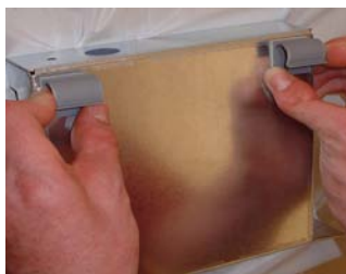
Figure 2-34. Affix cable clips.
