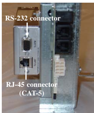
Figure 2-33. External Ethernet mounted (side view).
