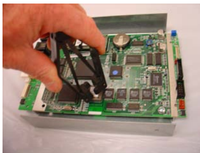
Figure 6. Remove Eprom chip.
