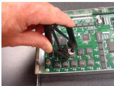
Figure 6. Remove Eprom chip.
