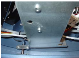
Figure 14. Route ribbon cable under Docking board bracket.
