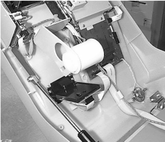
*Figure 6-4A. Paper Spool in its normal operating position.*
