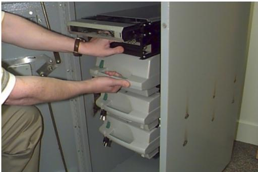
Figure 4-17a. Removing the Reject Cassette.
