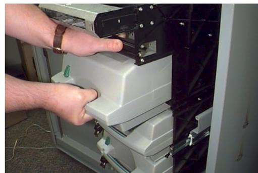
Figure 4-17b. Removing the Reject Cassette.
