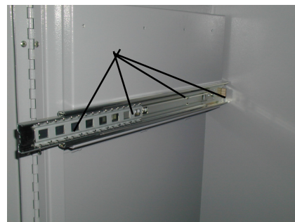
Figure 3. Screw location for slide rails.
