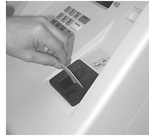
Figure 6-8. Use the cleaning cards on a monthly basis to maintain effective card reader operation.
