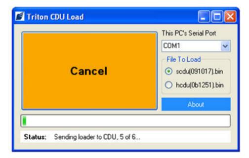
8. When the program has loaded completely, the status bar at the bottom will state Success. The dispenser can now be disconnected safely. Unplug the download data cable from the dispenser and reattach the unit's data cable.
